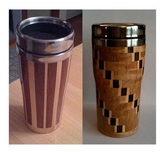
This is a fun project that is not nearly as difficult or complicated as the following procedures may suggest. The mug on the left is made from staves and follows the method that is most often seen in the literature (see references). It can also be made from a single piece of wood. Unless you are very experienced with staves and hollowing deep vessels, I would not suggest you try this. The mug on the right, however, is much easier to make and can be made with an infinite variety of patterns.
