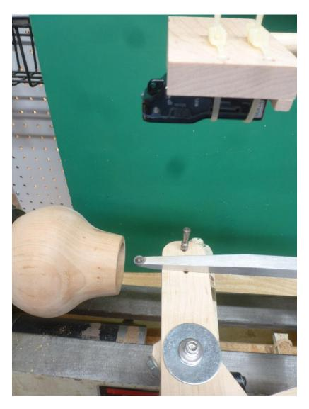
With the camera mounted directly over the end of the tool, the image that is sent wirelessly to the video display will always remain the same. That is, the end of the tool will always be in the same position relative to the camera image.
