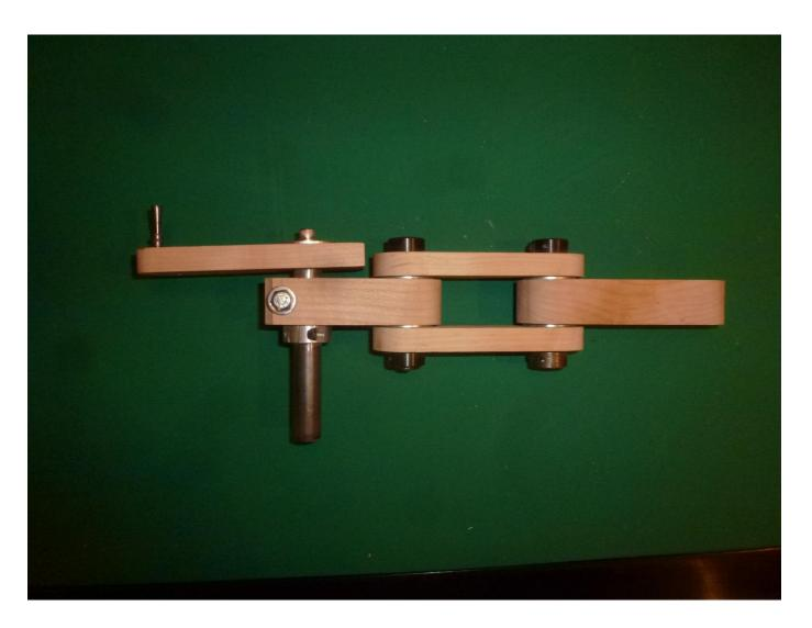
The replica arm assembly, with pivot posts, thrust washers and clamps providing the elements of the four bar linkage.
