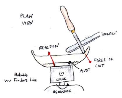
"...the problem of internal dovetail chucking having a tendency of splitting the recess out."
