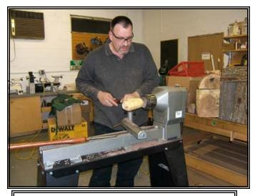
Here, Peter is taking off the top of a demo piece to finish up the inside and make a lip for the new lid to fit into.
