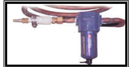
The copper condensing coil and the water trap are useful to dry the air from your air compressor.
