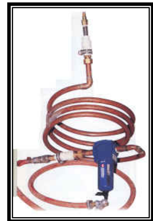
The condensing coil and water trap. Air from the air compressor goes through this coil which is sitting in water to cool it. Water condenses out at the bottom and the dry air goes to the steel pipe to be heated.
