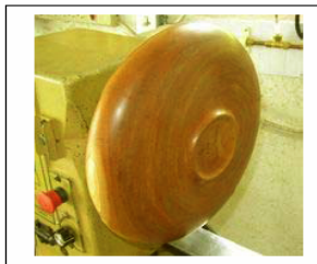
12 Inch Bowl Secured on 6 1/2" Chuck
