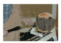
Once the outside of the bowl is round Ron increases the speed of the lathe and starts working on shaping the foot of the bowl which when completed he will attaché another faceplate to so he can turn the bowl around and begin working on the inside of the bowl. It is critical that the bottom be flat and sized properly so when you attach the faceplate it is a good solid fit.
