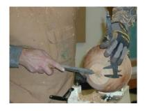
Here Ron is turning the inside of the bowl staring in the middle and working his way out and down. Once he has a consistent thickness from top to bottom he uses a jam chuck to clean up the bottom of the bowl as that is a key area that needs attention to detail to finish up the piece. Great looking Cherry bowl!
