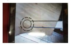
With the camera mounted directly over the end of the tool, the image that is sent wirelessly to the video display will always remain the same. That is, the end of the tool will always be in the same position relative to the camera image. Below is Ralph's homemade version. Note the camera is directly over (and follows) the cutter.
