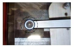
Secure a sheet of clear acetate to the face of the visual display (iPad) onto which you will draw the shape of the tool holder and cutting edge with a black Sharpie or Dry Erase marker.
